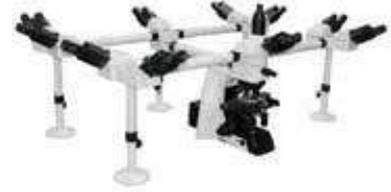
Multi Head attachment for 2/3/5/10/20 viewers, Main Observer sidentopf Trinocular Head/ inclined at 30°, FOV 25mm, rotating 360°, IPD 48-76, Binocular Head for Secondary Observation, inclined at 30°, Eyepieces 10X, upto 25mm, Side by Side Observation Head- 4Nos, multi color LED pointer, 360° rotatable, moveable with joystick, intensity adjustable
