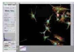
In fluorescence imaging, most area of the image is dark. In such case, the white balance is not able to give the correct color reference for the images. How can you do the color correction for the images? Black Balance helps you solve this.
